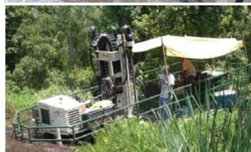
This setup has been extensively used in south Louisiana for exploration work associated with bridges, pipelines, levees, etc. We have performed CPTs and soil borings from marsh buggies to depths over 100 feet.
